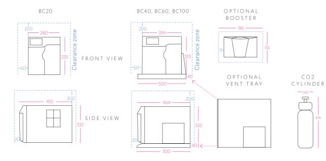
For full installation details please refer to the installation instructions which can be found at zipwater.com Be sure to allow additional space required if installing a sparkling model with CO2 cylinder.
